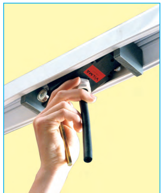
Fig. 3 - Extracting and replacing the trolley-collector.
